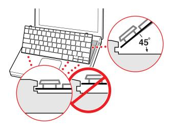
Pull down on the keyboard release tabs and then press down on the top portion of the keyboard.
