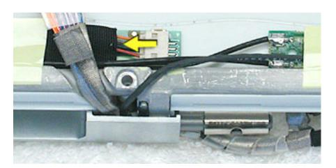
6. Remove the reed switch cable assembly.
