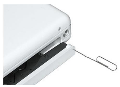
8. Warning: Avoid pressure on the optical drive tray. When removing the optical drive bezel, putting pressure on the drive tray can damage the drive.
