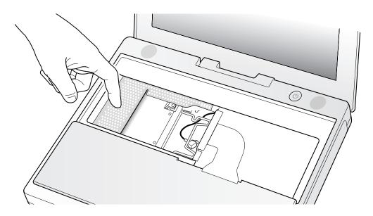
2. Unlatch the flexible wire holder that secures the card.
