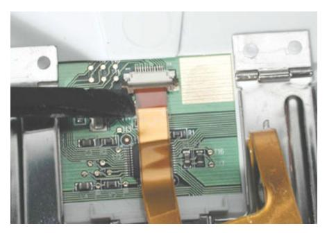
4. Holding the top case steady, press the latch in and over the lip of the top case. You might need to flex the latch opening somewhat to remove it from the top case.
