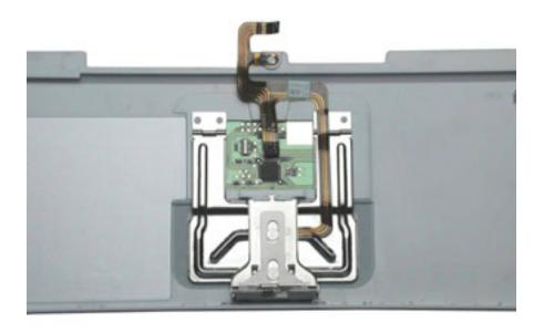
3. Use a black stick to lift up the ends of the connector that holds the trackpad cable to the board.
