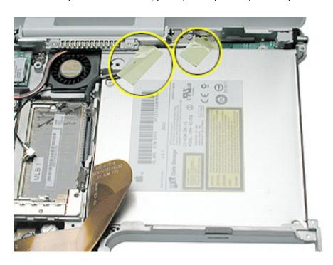
2. Remove the two screws from the tabs at the upper left area of the optical drive.
