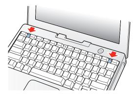
4. Flip the keyboard over and lay it on the palm rests and trackpad.
