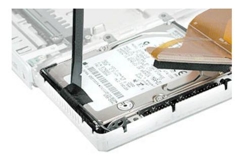
4. From the corner bracket, tilt up the hard drive, and slide it out from under the microphone cable.
