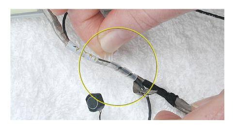
6. Remove the microphone cable from the assembly.
