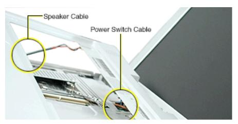
14. With the top case loosened, note how the speaker cable is routed.
