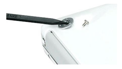
6. Remove the two identical Phillips screws next to the battery connector.
