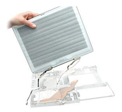
7. Warning: While supporting the display, do not tug on the remaining cables. Make sure the cable insulation is not torn or damaged.
