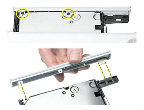
• For a combo optical drive, use the pointed end of a black stick to press the recessed middle of the thin tab. Then press the wider tab, and hold the drive tray steady as you pull the bezel off of the tray.
