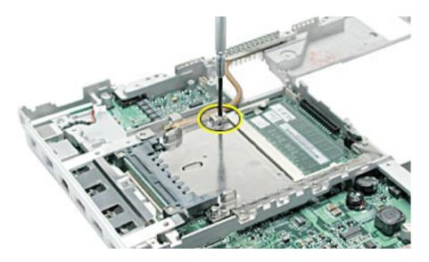
6. Tilt up the heat spreader and lift it off the logic board and out of the frame.
