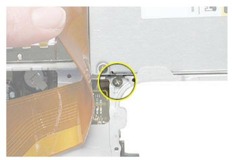
4. Warning: Handle the optical drive at the sides only. Do not touch or press anywhere else on the drive.
