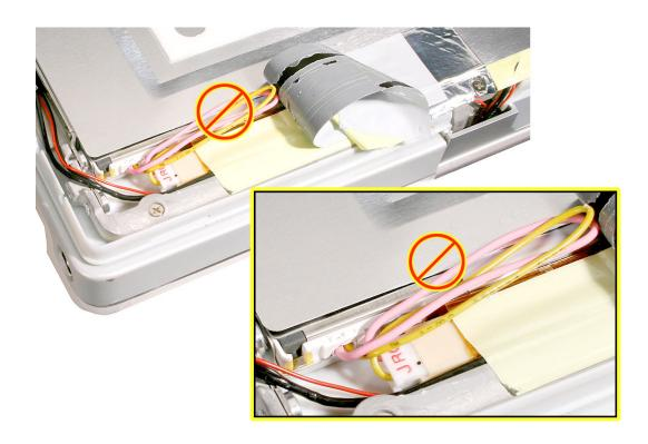
With the shield installed over the replacement LCD panel, apply a rectangular piece of foil tape to overlap the shield and cables at the left side of the clutch, as shown below.
