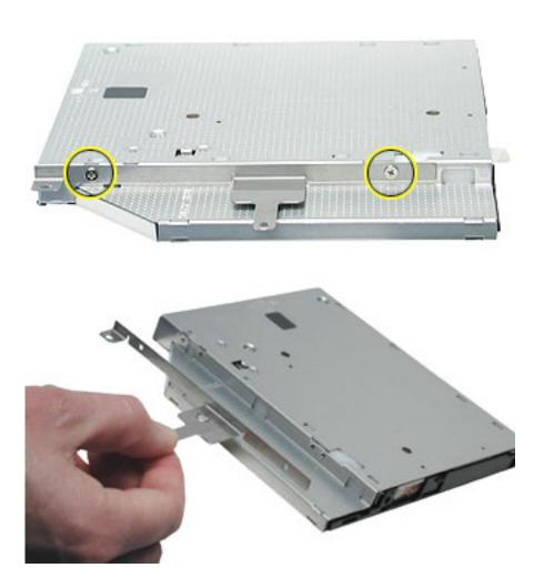
9. Install the replacement optical drive, and reassemble and test the computer.
