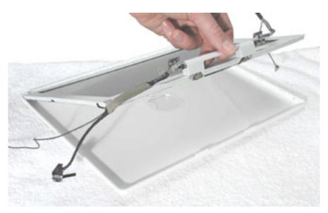
4. Place the display assembly face down on a soft cloth.
