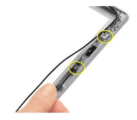
6. Tilt up the antenna receptor to remove it from the bezel assembly.
